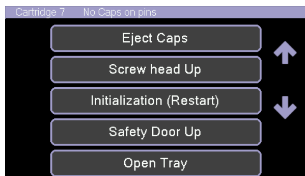
Figure 7-1: Manual Recovery Screen
